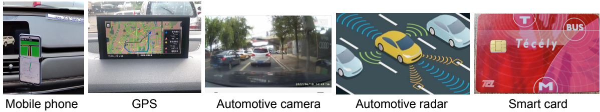
Figure 2.2: Off-roadway sensors reside on the moving objects. As shown above, pictures are taken or generated ourselves. They can record the trajectories and status of objects.
